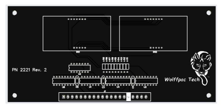
Insert U1 (74HCT02) into the board from the top side (the side with the lettering) so that one pin goes through each hole at the location labeled 'U1'. Each chip is marked with a 'U'-shaped notch on one of the short ends:
