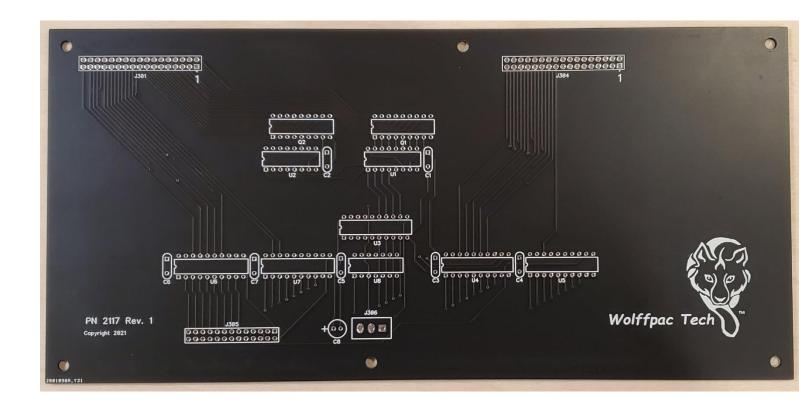
Insert U8 (74ACT32) into the board from the top side (the side with the lettering) so that one pin goes through each hole at the location labeled 'U8'. Each chip is marked with a 'U'-shaped notch (or dot) on one of the short ends:
