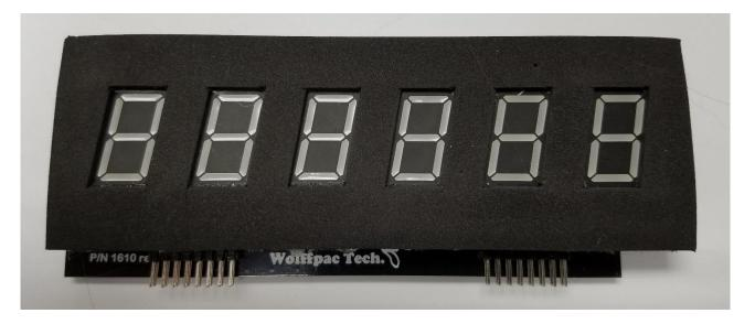
Step 4. Insert board 'B' (1620) with the LED's into the 'A' board (1950). Line the pins from J4 and J5 with the holes in J2 and J3 with the LEDs pointing outwards. Press down firmly. About 1/8" of board B should slide behind J2 and J3.
