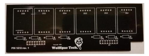
Step 2: Locate resistors R10-R16.
