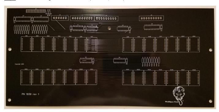
Insert U4 (74HCT32 or 74ACT32) into the board from the top side (the side with the lettering) so that one pin goes through each hole at the location labeled 'U4'. Each chip is marked with a 'U'-shaped notch on one of the short ends:
