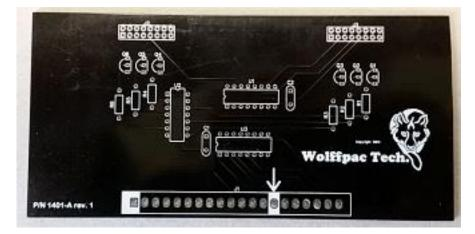
Insert U1 (ULN2003) into the board from the top side (the side with the lettering) so that one pin goes through each hole at the location labeled 'U1'. Each chip is marked with a 'U'-shaped notch on one of the short ends:
