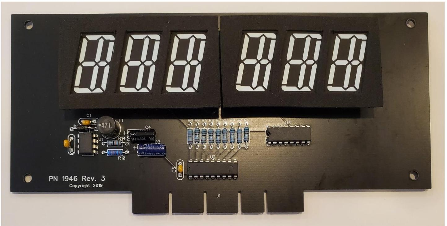
Step 3. Once the displays are dry, install the display in your pinball machine with the power off and attach the original cables. Apply power and enjoy!
