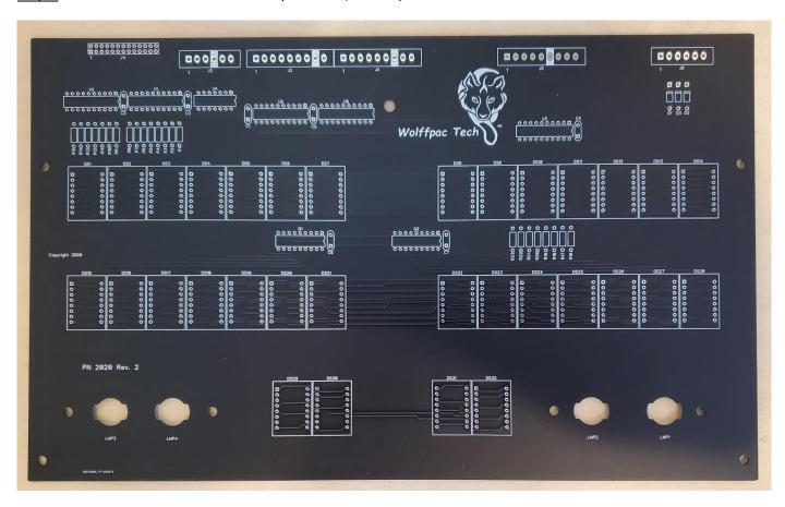
Insert U4 (74HCT32 or 74ACT32) into the board from the top side (the side with the lettering) so that one pin goes through each hole at the location labeled 'U4'. Each chip is marked with a 'U'-shaped notch on one of the short ends:
