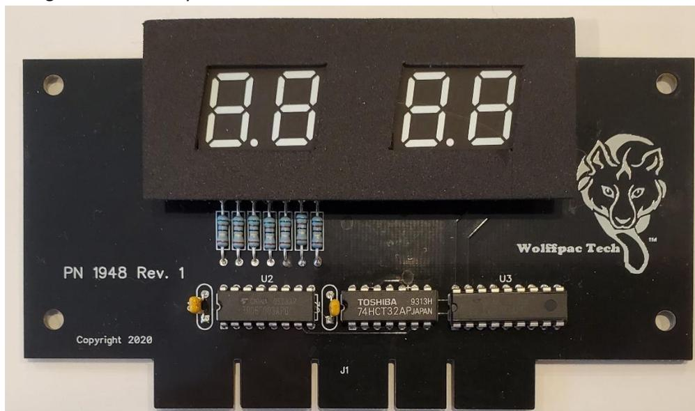
Step 4. install the display in your pinball machine with the power off and attach the original cable. Apply power and enjoy!
