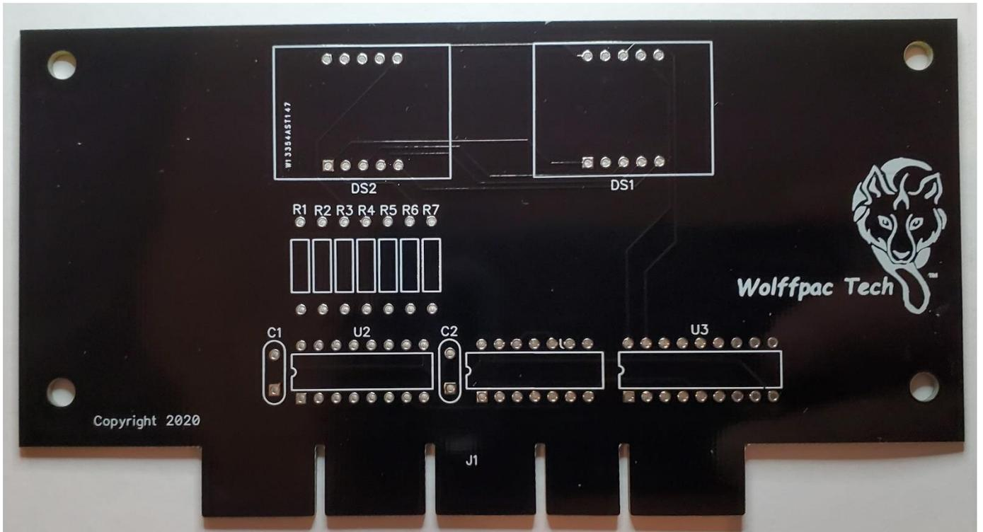
Insert U1 (74HCT32 or 74ACT32) into the board from the top side (the side with the lettering) so that one pin goes through each hole at the location labeled 'U1'. (Note: the marking 'U1' may be hard to read.) Each chip is marked with a 'U'-shaped notch on one of the short ends:
