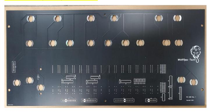
Insert U4 (74HCT32 or 74ACT32) into the board from the back side (the black side) so that one pin goes through each hole at the location labeled 'U4'. Each chip is marked with a 'U'-shaped notch on one of the short ends:
