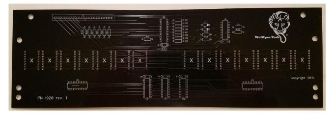
Insert U1 (CD4042) into the board from the top side (the side with the lettering) so that one pin goes through each hole at the location labeled 'U1'. Each chip is marked with a 'U'-shaped notch on one of the short ends:
