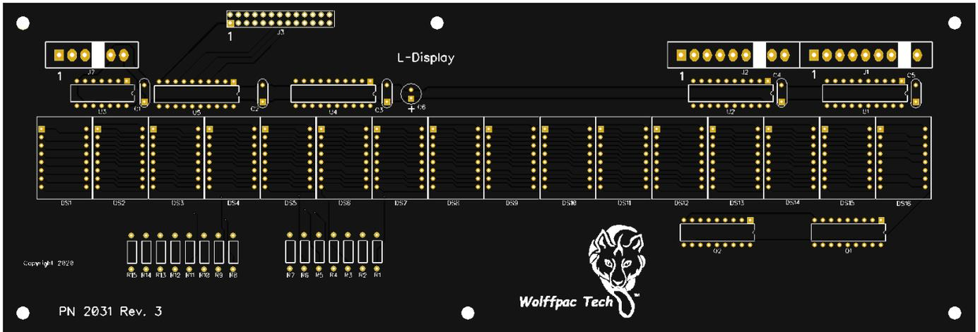
Insert U3 (74ACT08) into the board from the top side (the side with the lettering) so that one pin goes through each hole at the location labeled 'U4'. Each chip is marked with a 'U'-shaped notch on one of the short ends:
