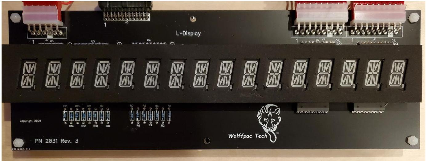
Step 6. With the power off, install the displays in your pinball machine and attach the original cables.
