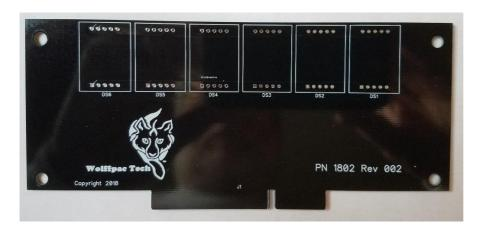
Step 2: 7-Segment LED's. The 7-segment LED's are installed in positions DS1-DS6.
