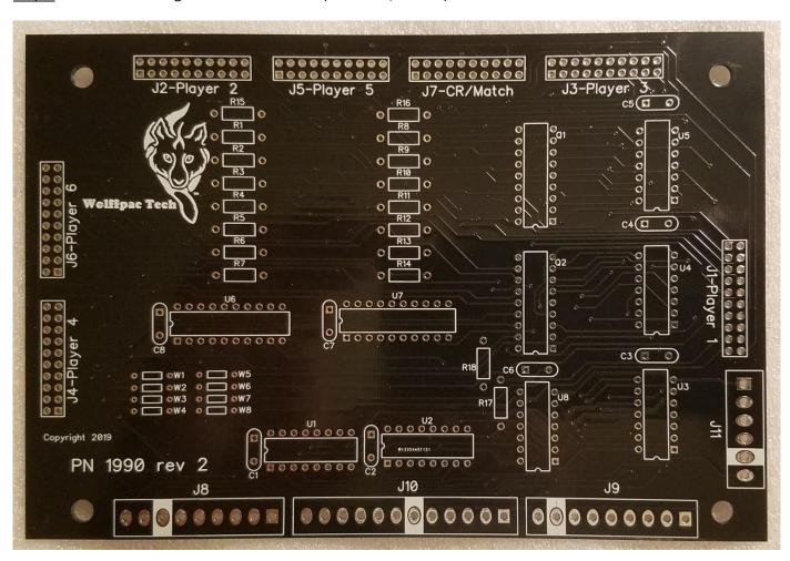
Insert U1 (CD4543) into the board from the top side (the side with the lettering) so that one pin goes through each hole at the location labeled 'U1'. Each chip is marked with a 'U'-shaped notch on one of the short ends:
