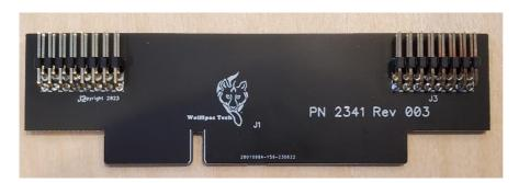
It is important that the connector is seated flush against the top of the board with the pins parallel to the board as shown:
