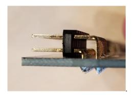
For this reason, it is recommended that you solder only one pin on each end of the header until you can confirm that the connector is seated flush and square with the top surface of the board. If not, you can reheat the pin while pressing on the connector from the opposite side. Solder the remaining pins in place.
