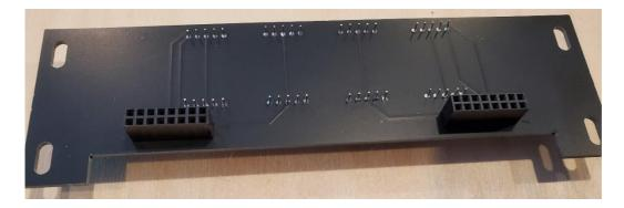
Insert one of the black, female 2x8 headers into the position marked J2 <u>from the back side of the board</u>. Make sure that all pins are correctly inserted through the holes.
