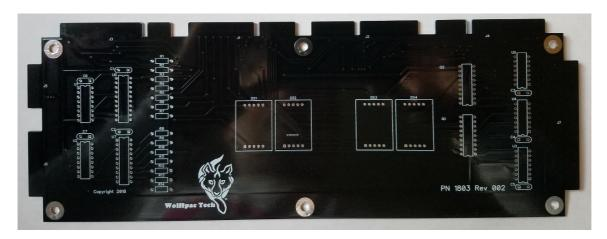
Insert U1 (CD4543) into the board from the top side (the side with the lettering) so that one pin goes through each hole at the location labeled 'U1'. Each chip is marked with a 'U'-shaped notch on one of the short ends:
